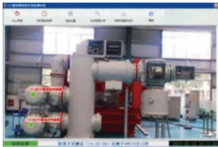
GIS partial discharge online monitoring (with main interface display)
